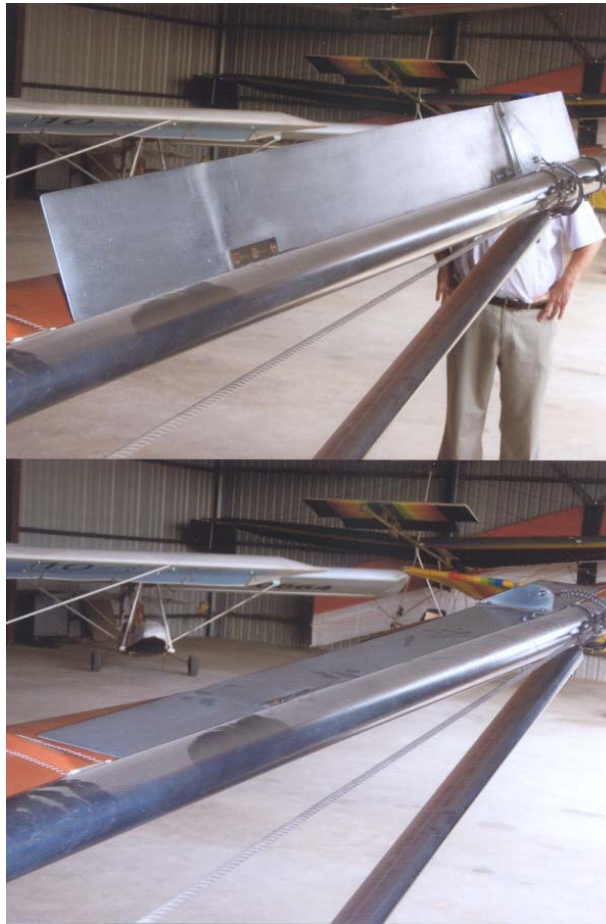
Top picture: Spoiler raised, drag increases, wing drops Bottom picture: Spoiler normal, wing level or rises if other spoiler is raised
