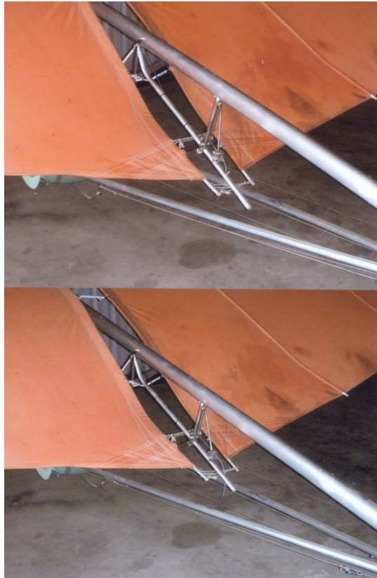
Top Picture: Trailing edge lowered, Drag and Lift increase, airspeed decreases for landing Bottom picture: Trailing edge raised, drag decreased, airspeed increases for cruising
