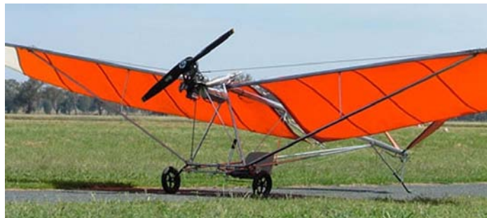
Note aluminium spars (struts) supporting the wings
