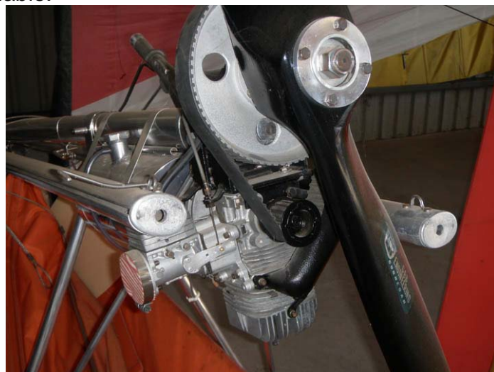
Note belt drive between motor and propeller shaft
